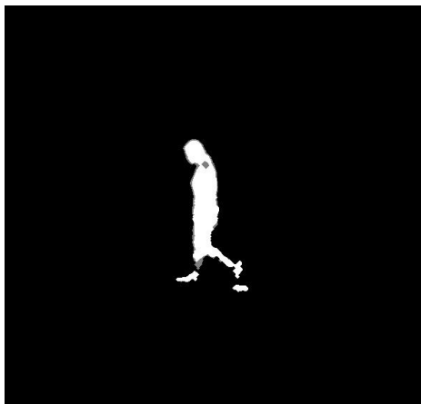
Binary image of moving object in frame
